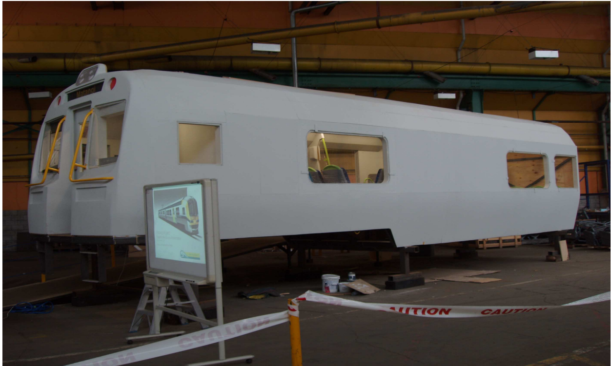
Figure 4. The wooden 'mock-up' of half of the low floor trailer car at the Hutt Workshops
