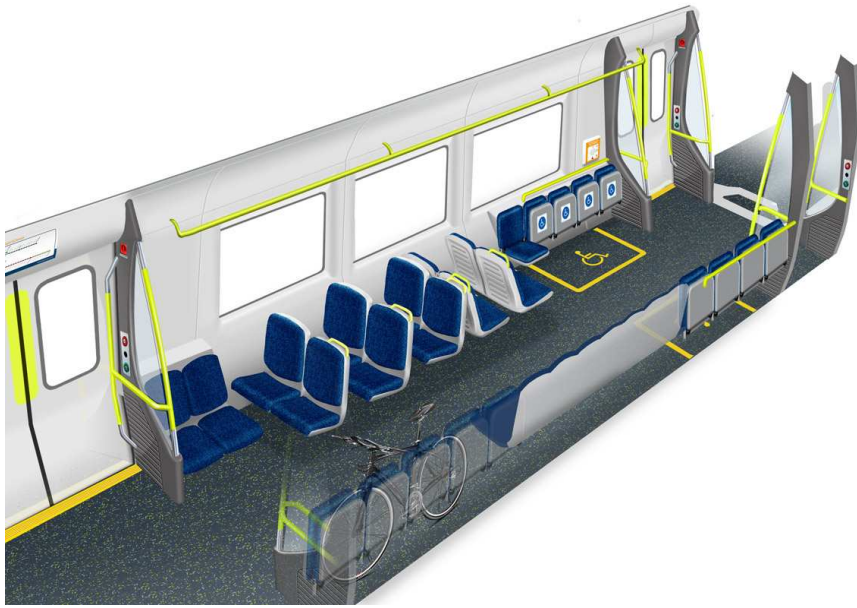
Figure 2. Trailer Car (low floor area) note lack of steps at doorways
